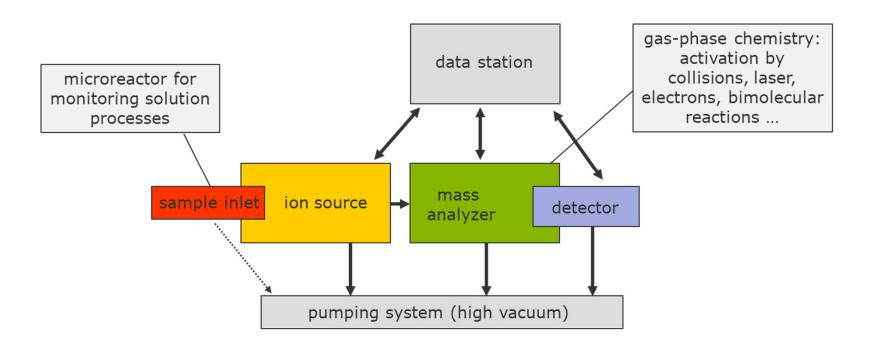
mass spectrometers are operated at pressures  $< 10^{-8}$  mbar
